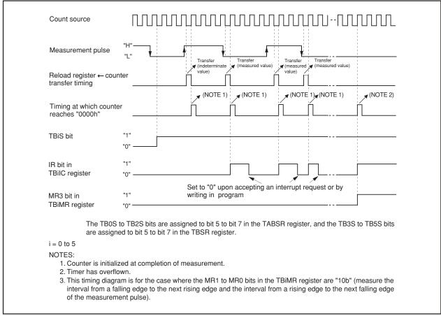
Figure 12.22 Operation Timing When Measuring Pulse Width
